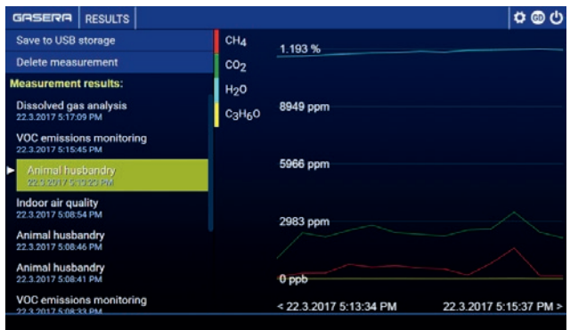
Figure 36. Results view with list of measurements. Preview of highlighted measurement is shown.
