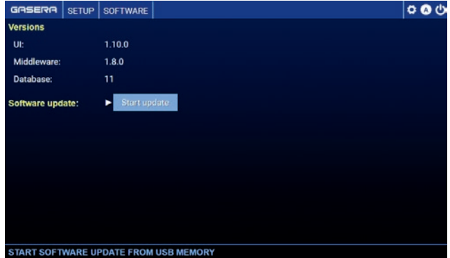
Figure 84. Starting the software update from the Software view in the Setup menu.
