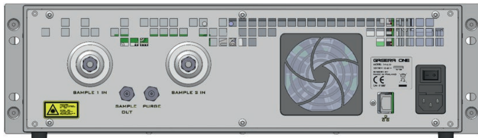
Figure 3. Rear view of GASERA ONE PULSE is shown above. The gas connectors are in the left side of the rear panel. The Ethernet connector, mains connector and power switch are on the bottom right corner. GASERA ONE FORMALDEHYDE and GASERA ONE SHED slightly different positions for the fan and the gas ports.
