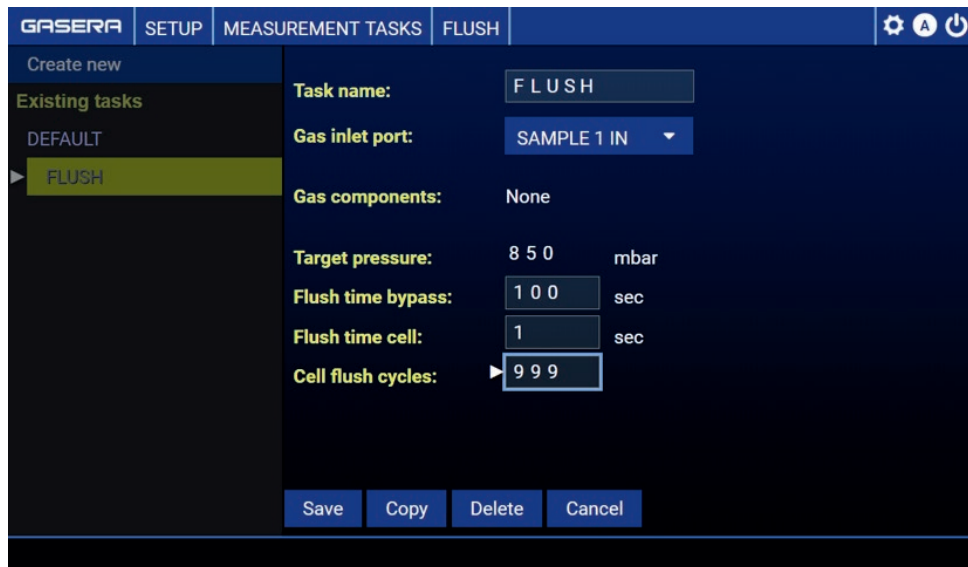
Figure 56. Measurement task for Flushing operation.
