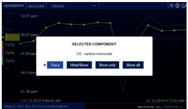
Figure 29. The trend view pop-up for tracing, hiding or showing the selected analyte data.
