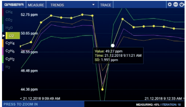
Figure 30. The trace shows values for the individual data points in the trend curve. Pressing the GASERA ONE Button will activate zoom in and zooming pop-up.
